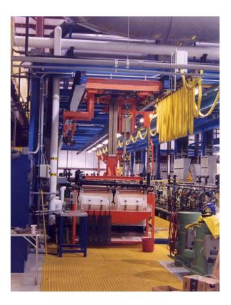
Hoist line will accommodate an extensive range of tank configurations including ultrasonics. All models include variable frequency motor controllers with adjustable acceleration and deceleration for smooth, controlled stops and starts. Traverse brake wear is virtually eliminated. Industrial proximity switches are controlled and monitored through state of the art PLC's for consistent station control.
