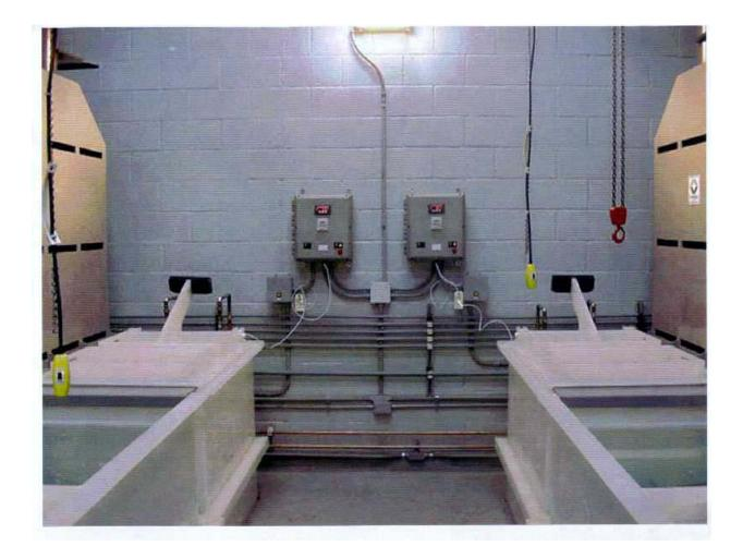
Installed in a turbine repair facility for processing high temperature alloys. Note the counterbalanced covers on acid processing tank to minimize fumes from hot  $(140^{\circ}F)$ concentrated Hydrochloric Acid
