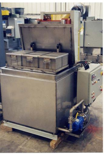
Up and down vertical motion provides vigorous agitation to remove chips, oils, buffing compounds, and greases. Stroke and speed are adjustable to provide aggressive cleaning for difficult parts or gentle action for delicate parts.
