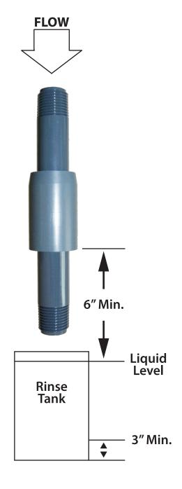
This device surpasses recognized national standards for vacuum breakers when installed as illustrated.
