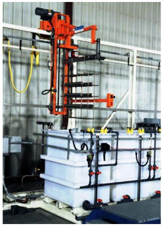
Hoist line will accommodate an extensive range of tank configurations including ultrasonics. All models include variable frequency motor controllers with adjustable acceleration and deceleration for smooth, controlled stops and starts. Traverse brake wear is virtually eliminated. Industrial proximity switches are controlled and monitored through state of the art PLC's for consistent station control.
